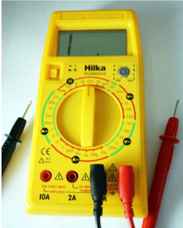
Picture 7: Multimeter settings to check motor readings
